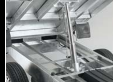
Large 3-stage tipping cylinders
