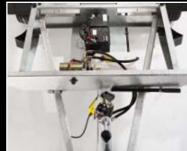
combined operation of hand and electric pump
