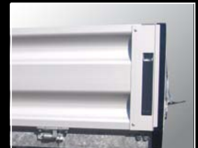
side wall 350 mm (fitted)
