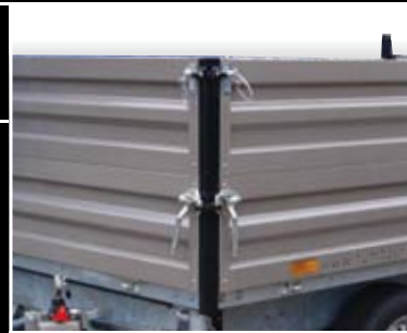
side wall extension steel, 350 mm rear swinging
