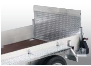
Sturdy aluminium mudguards fold up automatically when lowering
