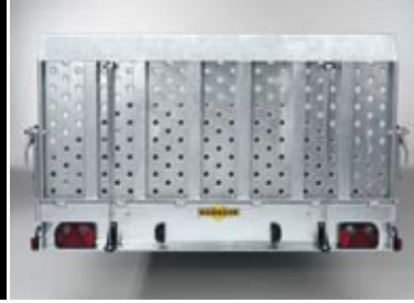
Perforated drive-over strip folded up with gas-spring support
