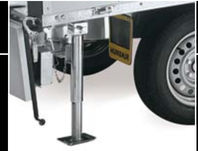
telescopic crank supports (2 pieces)
