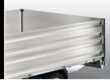
Optionally available with 350 mm high side wall extensions
