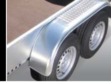
Hot-dip galvanized steel mudguards covered with aluminium chequer plate, that can be stood on
