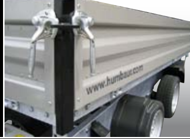
Side walls made of galvanized and powder-coated steel
