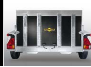
Access flap made of wood and drive-over wedge made of aluminium
