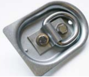
lashing rings flush-mounted in wooden floor, pull force each 0.4 to (4 or 6 pieces)
