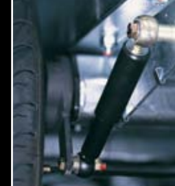
Wheel shock-absorbers (for 100 km/h approval)
