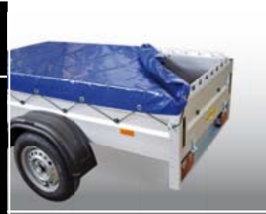
flat tarpaulin version with railing at the side (including railing front + rear)
