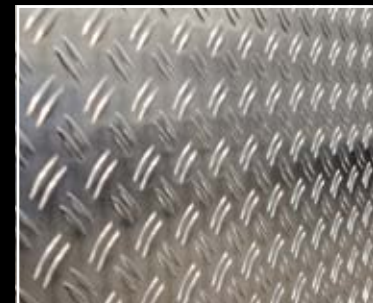
floor plate covered in aluminium chequer plate
