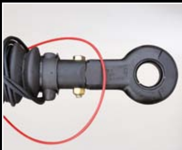
DIN towing eye for HV drawbar, 2000 kg–2500 kg, 2000 kg–2500 kg and 3000 kg–3500 kg
