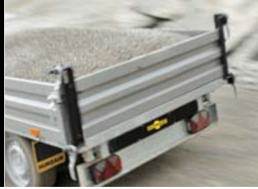
Solid underguard with integrated lighting unit
